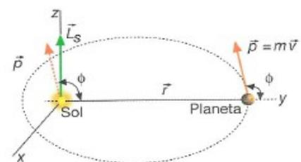
$$\text{si } \vec{r} \parallel \vec{F} \Rightarrow \vec{M} = \vec{r} \times \vec{F} = 0$$
