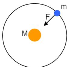
$$\left. \begin{aligned} F_c &= m a_N \\ F &= G \frac{m M}{d^2} \end{aligned} \right\} \Rightarrow a_N = G \frac{M}{d^2}; \quad a_N = G \frac{M}{d^2}$$
